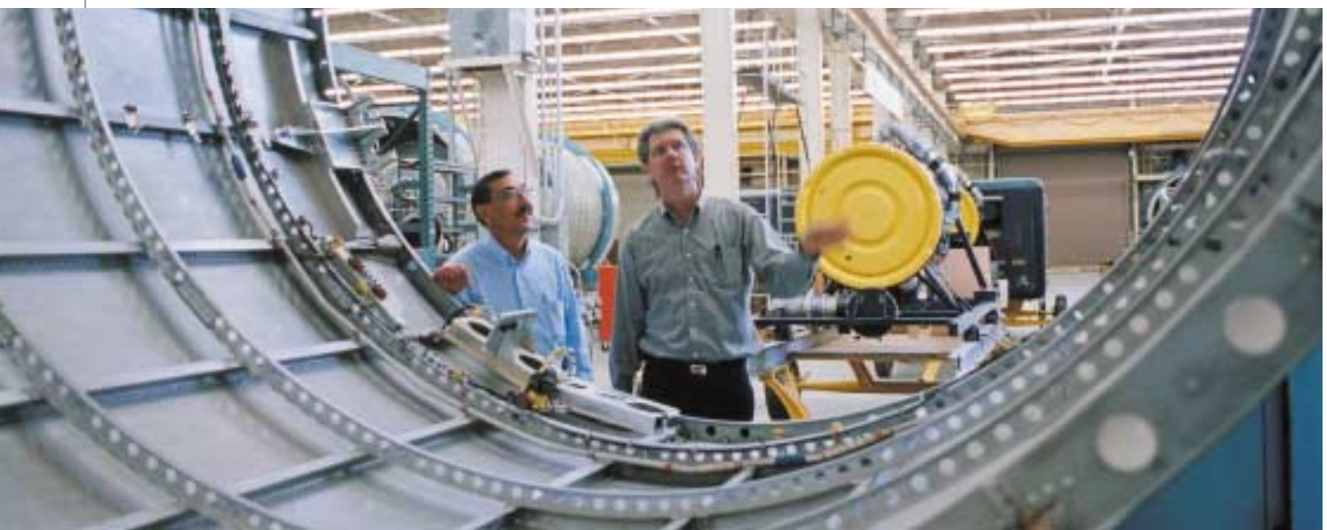
AN INTERSTAGE SKIRT, WHICH JOINS THE FIRST AND SECOND STAGES OF A TITAN II BOOSTER, UNDERGOES INSPECTION. AEROSPACE WORKS CLOSELY WITH CONTRACTORS THROUGHOUT THE LAUNCH PROCESS TO PROVIDE INDEPENDENT ASSESSMENTS FOR THE U.S. AIR FORCE, THE NATIONAL RECONNAISSANCE OFFICE, AND OTHER CUSTOMERS.
