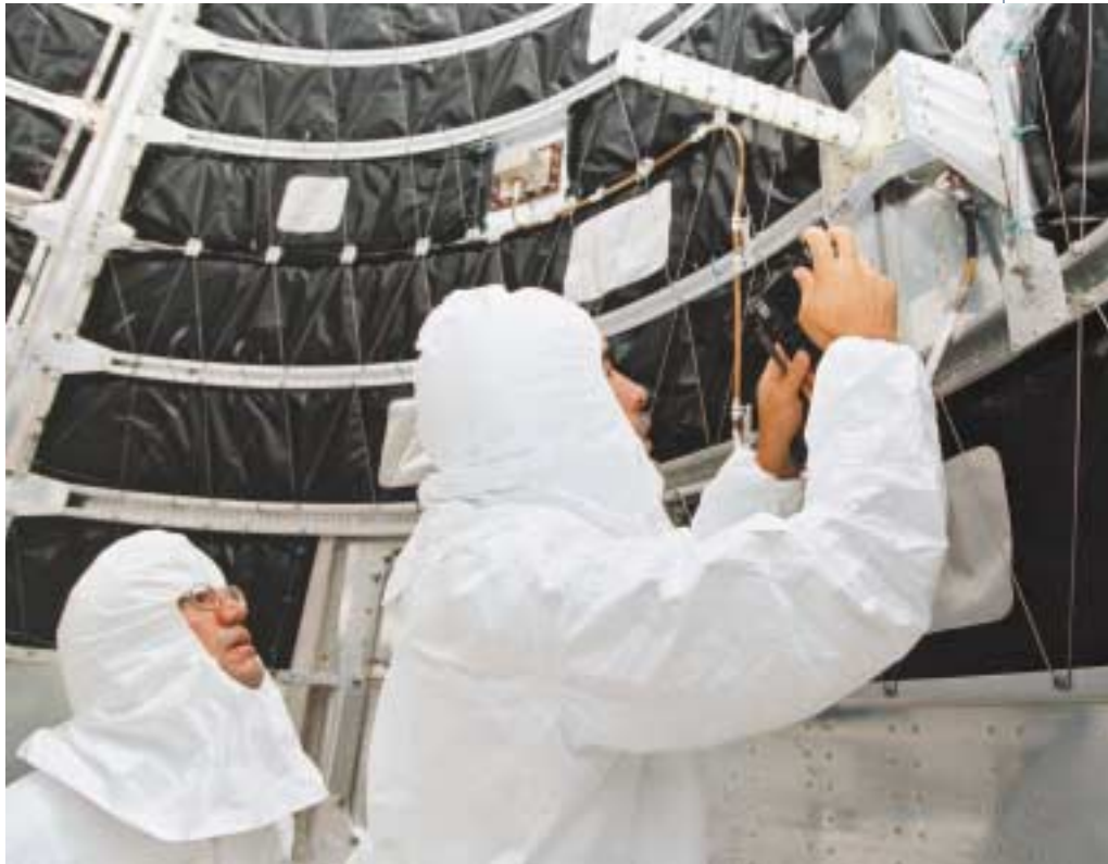
MEMBERS OF THE AEROSPACE TECHNICAL STAFF INSPECT THE FAIRING OF A TITAN II LAUNCHER TO ENSURE PROPER CLEARANCES FOR A DMSP PAYLOAD.
