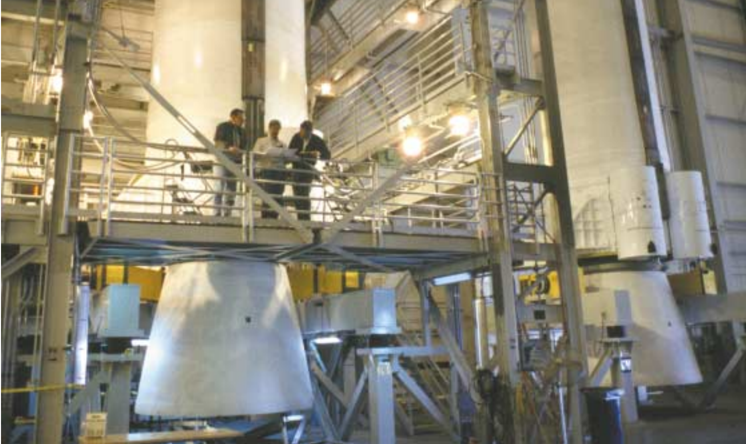
AEROSPACE ENGINEERS DISCUSS PROCEDURES WITH A CONTRACTOR IN THE SOLID ROCKET MOTOR PROCESSING FACILITY AT VANDENBERG AIR FORCE BASE. BEHIND THEM IS THE AFT SEGMENT OF A SOLID ROCKET MOTOR UPGRADE PLANNED FOR FLIGHT ON A TITAN IVB IN 2000.
