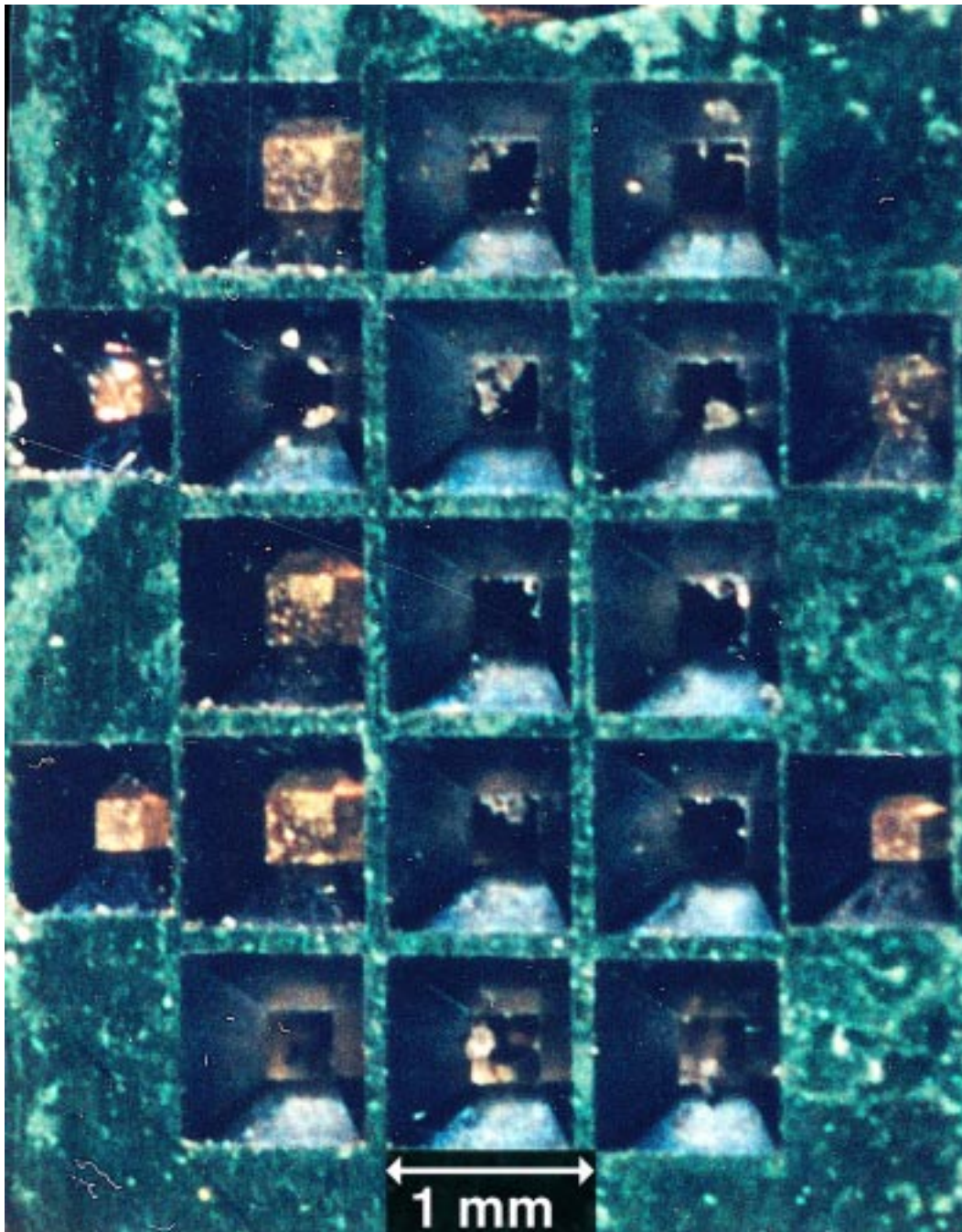
Figure 5: Digital Propulsion micro-Thruster chip, after firing in a vacuum. This image shows the central 3x5 array of thrusters, surrounded by 4 alignment holes. The center-to-center distance between the thrusters is 1 mm. Of the 15 thrusters, 12 fired successfully, and 3 did not fire (apparently, due to corona discharge effects in the firing circuitry). The 3 unfired thrusters are clearly visible: the brightly reflective intact burst diaphragms in the 1st, 3rd and 4th thrusters down in the left-hand column of the 3x5 array. The remnants of the ruptured diaphragms can be seen in the 12 fired thrusters.
