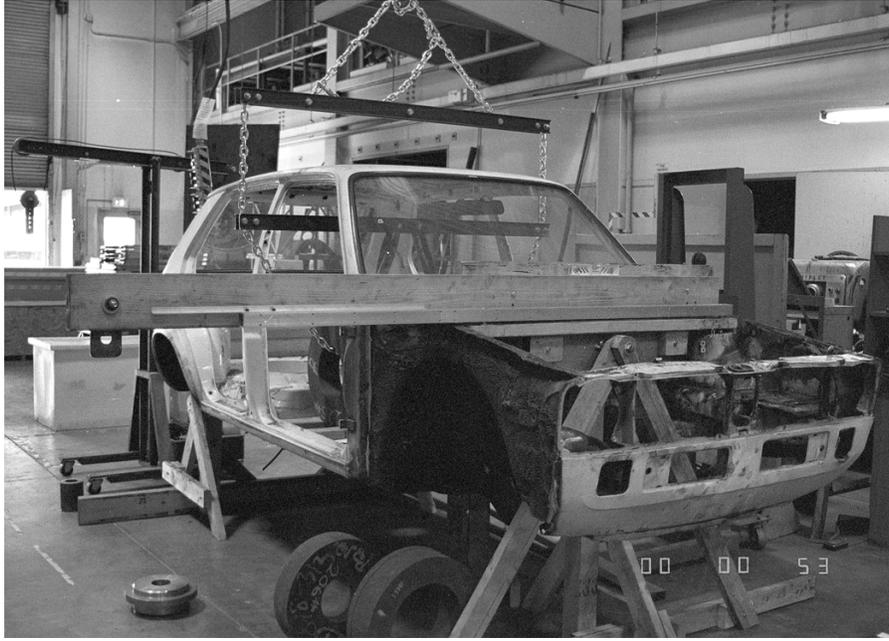
Figure 8.2 1980 VW Rabbit in Stiffness Testing
