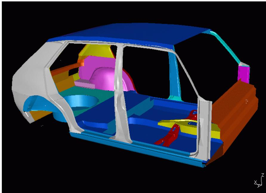
Figure 8.3 Geometric Model of Body-In-White in SDRC I-Deas
