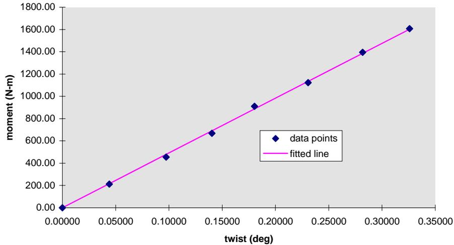
Figure A.1 Load Test, Torsional Stiffness
