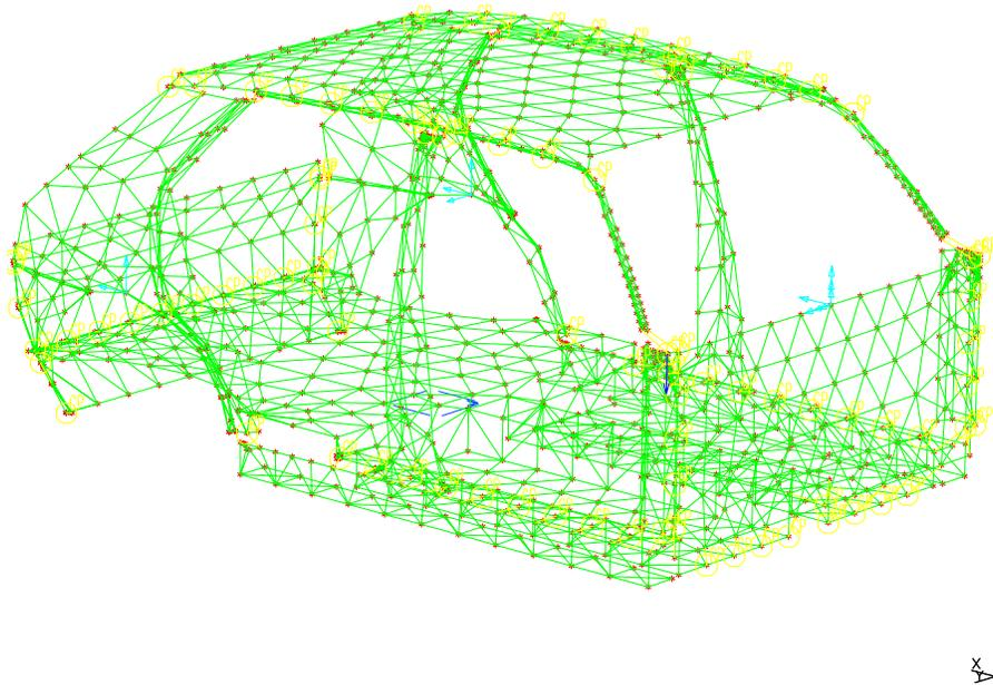
Figure 8.4 Finite Element Model of Body-In-White
