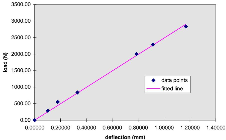
Figure A.2 Load Test, Torsional Stiffness
